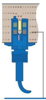
The robust Cambridge Viscosity oscillating piston system can measure a wide range of samples, including asphalt, lubrication oils, and heavy fuel oils, as well as handle any process upsets without damage to the system.
